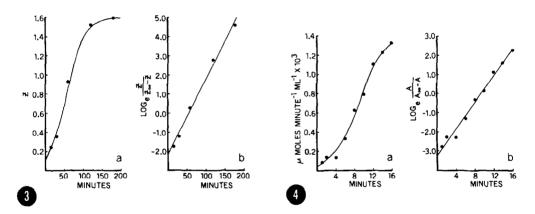
Figure IIIa shows the autocatalytic activation of C1s in the presence of added C1r. Z is the number of hemolytic sites generated in the C1s assay. The curve is calculated from the equation for an autocatalytic reaction where k =  $2.56 \times 10^{-2}$ ,  $A_{\infty}$  = 1.62 and  $A_{\alpha}$  = 0.139. The data are taken from (9).
